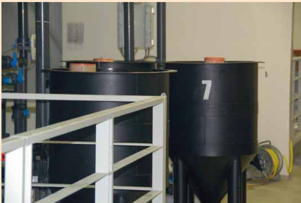
An incubation tank used to hold the eggs that are collected from the broodstock. After 4-5 days the eggs hatch and the larvae are moved to larval tanks.
